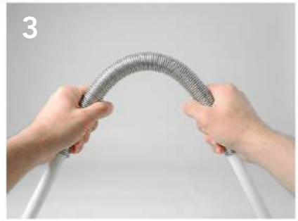
3 Use the Internal/External Bending Springs for bending the pipe to avoid dents
