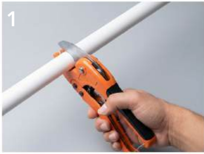
1 Cut the pipe from a perpendicular angle using the Pipe Cutter
