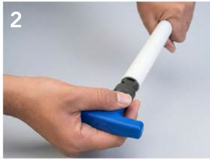
2 Round and chamfer the pipe using a reamer with 3-5 rotations for proper insertion
